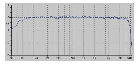
The bass frequency attenuation is caused by the microphone preamplifier circuit. The high end attenuation is caused by Sound Blaster 16 card. As seen in the measured performance, the microphone preamplifier is suitable for speaker measurements made using suitable measurement software and sound card. Using this preamplifier connected to line level input the problems caused by poor microphone preamplifier in many sound cards can be avoided.
